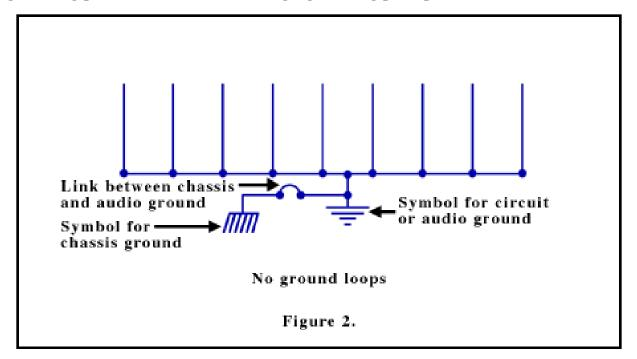
Figure 1 shows what not to do. If one connects an imaginary wire anywhere on the grid, one quickly sees that there are multiple paths to the symbol marking the ground, or in this case multiple grounds. Figure 2 shows only one path to ground from anywhere in the circuit. When designing and wiring a sound system, one needs to keep this approach in
