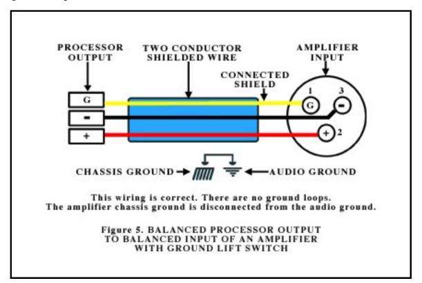
Cutting the shield at the amplifier end, prevents a ground loop from being created with two wires (perhaps of different gauges) being connected between two points.
